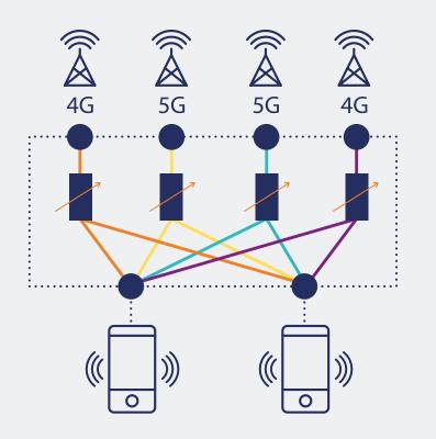
A handover test system is able to attenuate the signal from a simulated user equipment device, which simulates fading characteristics and can be used in the development of base station software and other aspects of wireless network handover activity.
