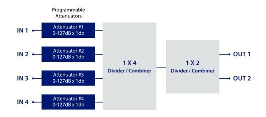
Full fan-out, bidirectional handover test system is capable of presenting each input to each output simultaneously in both the forward and reverse directions, while a limited fan-out, undirectional handover test system can only present an input at each specific output one-at-a-time and only in the forward direction.
