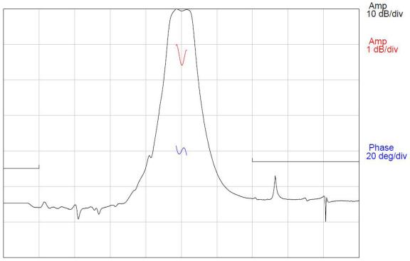
Center = 162 MHz, 0.2 MHz/div (2.5 kHz incr)
