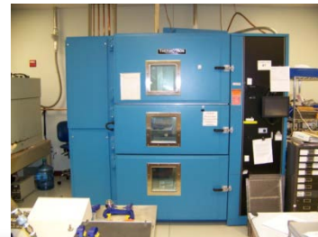
Extensive Burn-in and Thermal Cycling Capabilities
