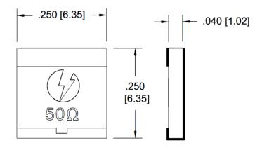
\*Dimensions are for substrate only and do not include terminal thickness or optional tinning thickness.
