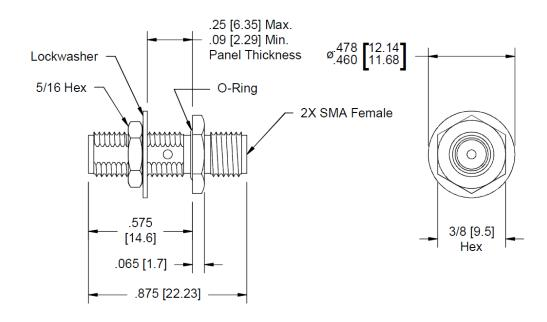
Panel nut, lock washer and O-ring are shipped unassembled.
