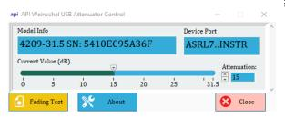
Spectrum Control 's Weinschel LabView based USB Control Center Software (AUCS) can also be used in the operation of this series of digital attenuators. The AUCS will allow the user to setup, control, and perform test and measurements over a standard USB 2.0 communication interface. Additional information is available in the Operating & Installation Manual, IM-611.
