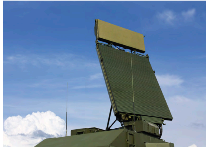
All-around antenna. Phased array technology.
