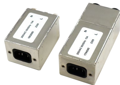
Two EMI filters. There is no way to tell by looking at them if they have built-in transient suppression.
