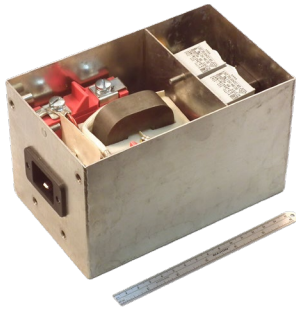
A 16A EMI powerline filter with transient suppression designed to meet MIL-STD-188-1 for HEMP protection. The entire filter would be about 80% smaller without the transient suppression.
